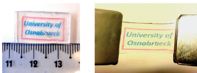
Figure 4. Photographs of an approximate 1-mm-thick elastomeric PDMS monolith containing micropatterns of embedded dye-containing microcapsules: (a) relaxed elastomeric PDMS monolith; (b) elastomeric PDMS monolith subjected to tensile stress.
